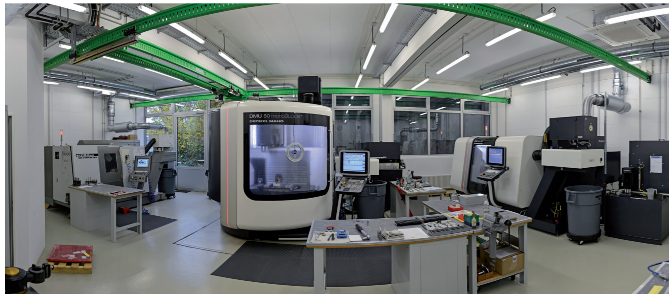
Panoramic view of the new workshop room equipped with the two CNC lathes (left CTX 320 and right CTX 800) and the CNC 5-axis milling machine DMU 80 Monoblock (center).
