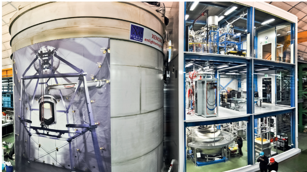
Fig. 3: The XENONIT experiment. On the left the water tank containing the xenon cryostat and on the right the service building with various auxiliary systems.
