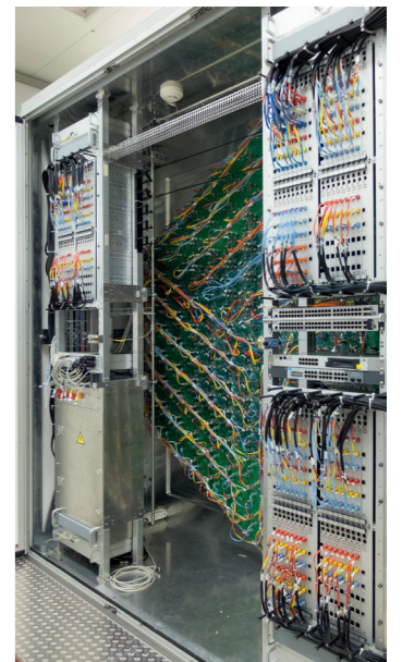
Fig. 10: Rear view into the FlashCam body, showing in the centre the photon detector plane modules, and in racks left and right the Flash-ADC modules and trigger processors.
